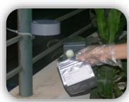
5. Place PS face down into a funel with the end attached into a GC vial. Shake so that charcoal falls down into the vial. Store the vial in zippered aluminium envelop.
