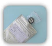
3. Attach passive samplers under shelter.
