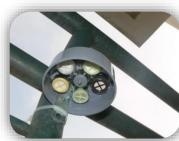
4. Place passive samplers back into envelop. Record the end of exposure.
